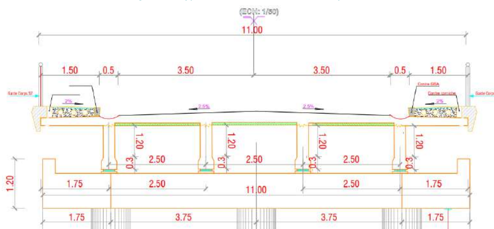
Figure 5 : Typical cross-section of deck on abutment
